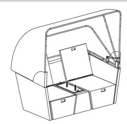
2 Move the centre table as shown to secure in position.
